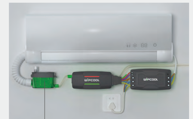
Failure drainage status-Output was cut off when water reaches alarm level to trigger safety switch, To prevent refrigeration equipment continues to generating the condensate water
